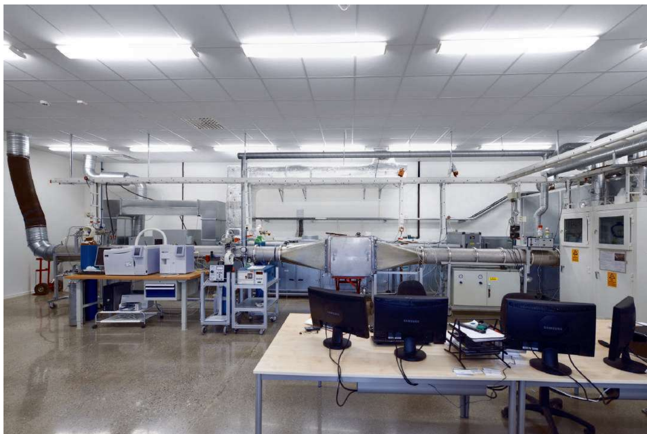
Molecular filter test equipment according to ISO 10121
